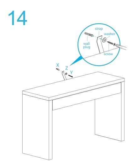
Attach 1x safety strap (V) to the top of the back side of the unit using 1x washer (Z) and 1x screw (W). Tighten with a screwdriver.
