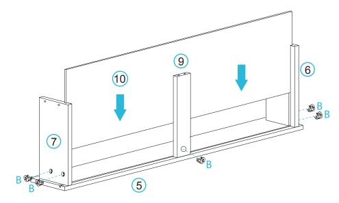
Attach panels [6], [7] and [9] by the bolts on panel [5].
