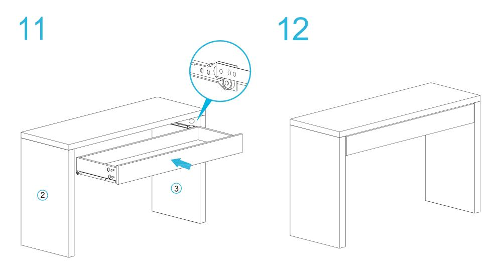
Insert the completed drawer into the desk, ensuring the rails are properly aligned and the drawer slides easily along.
